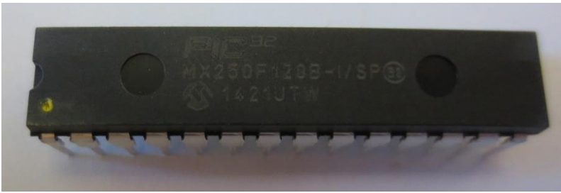
Figure 8 PIC32 MX250F128B in DIP-28 package
