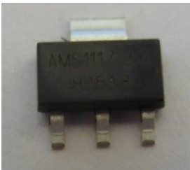
Figure 11 AMS1117 3.3V linear regulator
