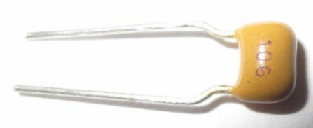
Figure 13 10uF tantalum capacitor
