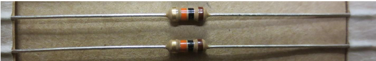
Figure 10 10k ohm resistor
